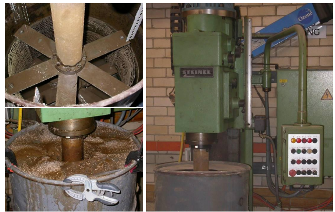
Figure 12. Application of wear treatment simultaneously to six netting panels. Top left - view of wear application wheel holding 6 net samples inside an empty grit slurry container. Right - milling machine used to rotate the wear application wheel. Bottom left - view of grit slurry container during the wear application process.
