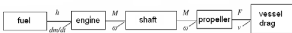
Figure 1: Representation of ship's propulsion system in bond-graphs with effort (above the arrow) and flow (below the arrow) variables.
