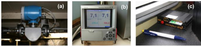
Figure 1. CorFu-m system mounted onboard the monitored semi-pelagic fishing vessels: (a) mass flow sensors for the measurement of fuel consumption; (b) multi channel recorder mounted on the vessel's bridge for the visualization of the fuel consumption; (c) GPS data logger.
