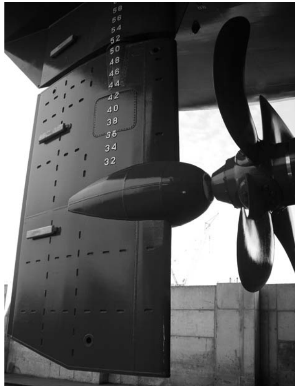
Figure 18. Twisted rudder designed by VICUSdt fitted on a vessel
